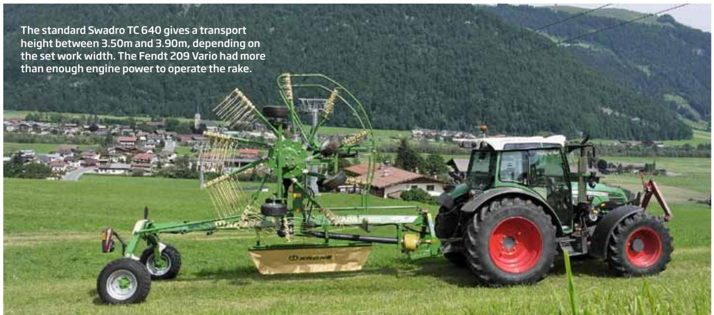
The standard Swadro TC 640 gives a transport height between 3.50m and 3.90m, depending on the set work width. The Fendt 209 Vario had more than enough engine power to operate the rake.
