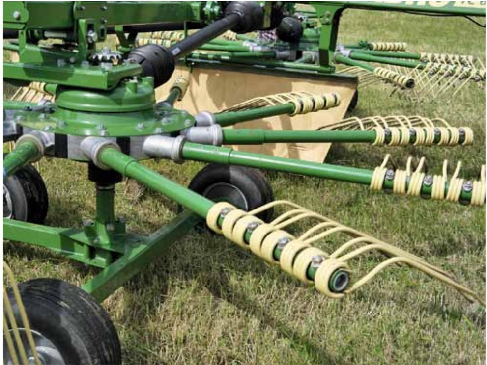
The fully-sealed bevel gearboxes and the tine arm bearings are lifetime lubricated. The bearings are made from robust cast aluminium and are connected gap-free with the arms.
