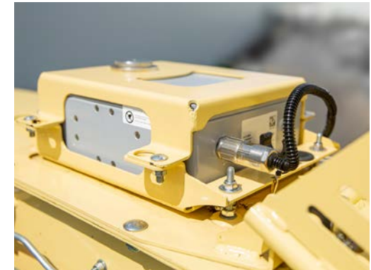
NIR sensors accurately measure nutrient and DM levels, allowing farmers to determine the optimum time of harvest.
