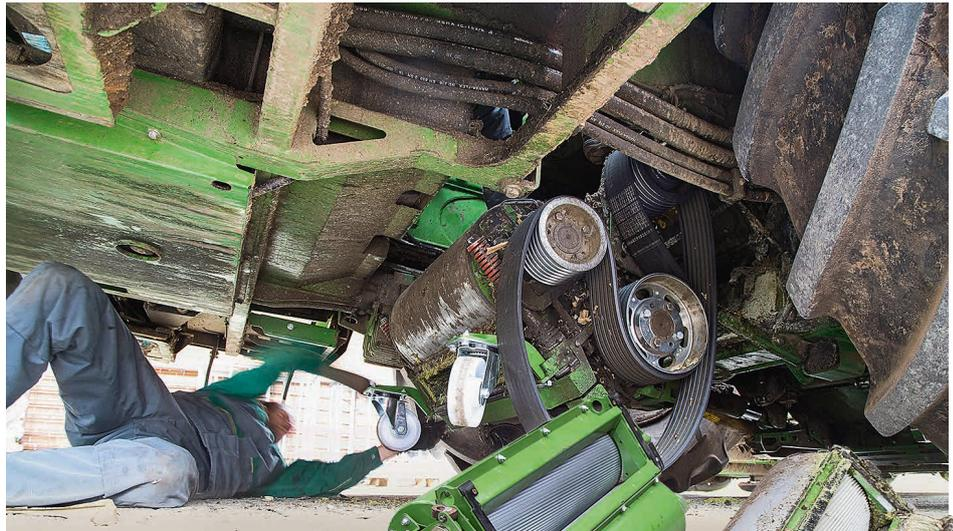
Swapping the cracker takes an hour after the rolls are clamped to the unit. Solid ground, such as concrete or tarmac, is a 'must'.
