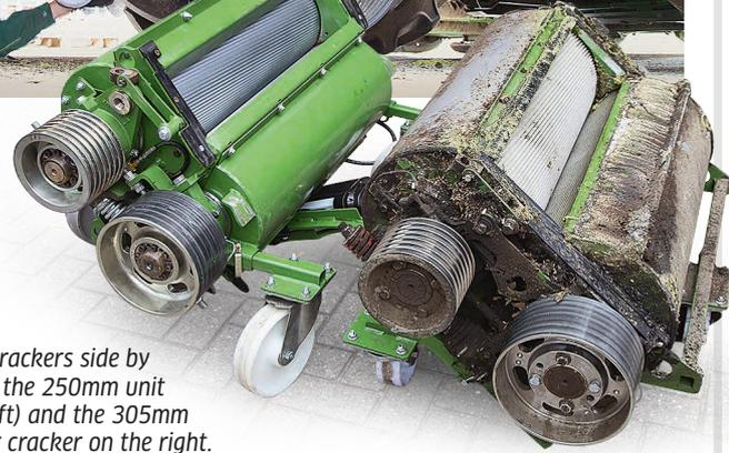
The two crackers side by side – the 250mm unit (left) and the 305mm diameter cracker on the right.
