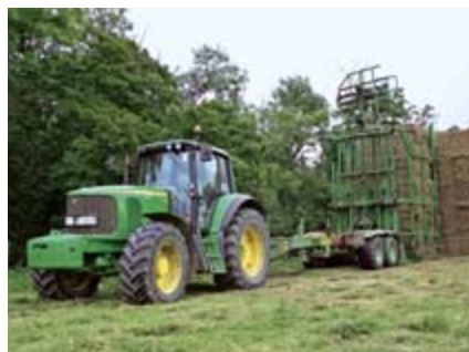
The Walton chaser is capable of handling the wide variety of bale sizes produced by the firm's four balers. It can shift about 700 bales a day.
