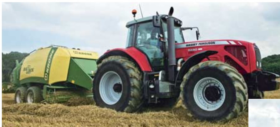
Fresh on the fleet this year, a 290hp MF 8480 pulls the new Krone Big Pack 1290 HDP. The Massey's stepless Dyna-VT gearbox is reckoned to make the big red tractor ideally suited to baling work.
