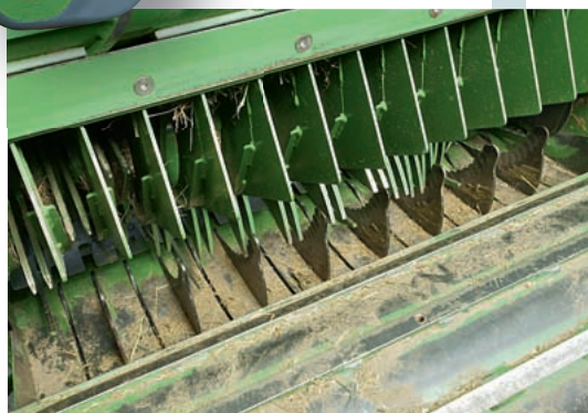
Comprima F155 XC has a 17-knife cutter (64mm chop). There is the option to spec a 26-knife system for a 42mm chop.
