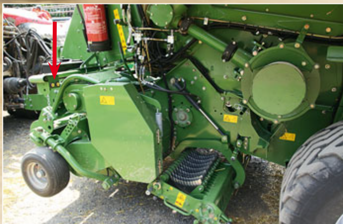
The knife drawer lowers via buttons (arrow). One half then pulls out to the nearside, the other to the offside. The big housing (right) covers the driveline protection clutch for the VFS packer.
