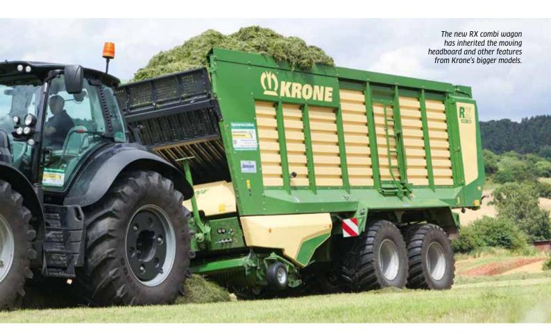
he new RX line-up comprises three models; the RX360 (36m<sup>3</sup>), RX400 (40m<sup>3</sup>) and RX430 (43m<sup>3</sup>), which all share the same chassis and body. The difference in capacity comes from the body: RX360 has a vertical headboard and back door; RX400 gains the pivoting front from the larger ZX wagons and an increase in capacity of 4m<sup>3</sup>; and, lastly, the RX430 gets its extra 3m<sup>3</sup> of storage capacity from a rucksack tailgate.
