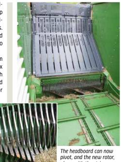
ne neadboard can now pivot, and the new rotor, along with the stripper fingers, is made from Hardox steel.
