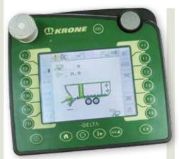
The Delta operator terminal is included in the base spec, while an ISObus version is optional and operated either via a CCI display or the tractor's own terminal.
