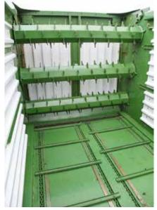
Chain/slat floor has four round steel chains and is powered by a pair of hydraulic motors with fast advance mode. GD models come with two rear beaters, but the majority of UK/Irish machines will be GL versions with no beaters.
