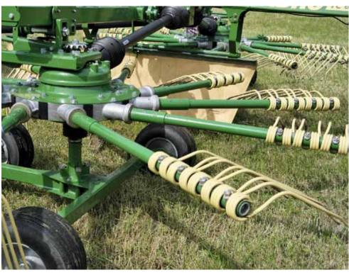
The fully-sealed bevel gearboxes and the tine arm bearings are lifetime lubricated. The bearings are made from robust cast aluminium and are connected gap-free with the arms.
