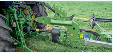
Our German spec machine had a top mount hitch, but this can be repositioned for lower mounting. A headstock for coupling to the lift arms is an option.
