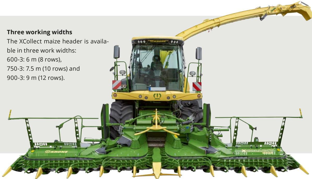
The three-section headers work to the well-proven EasyCollect collector principle. The XCollect splits the action of cutting and feeding into two separate processes.
