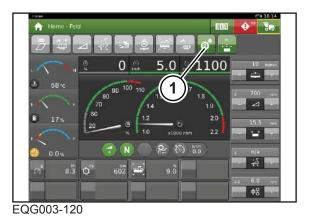
When the main coupling has been switched on, the machine control automatically detects the gearbox position of the VariLOC cutting length gearbox.
